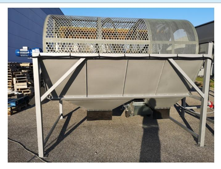
Rotating screen with drum length of 2-3 or 4 meters, screening mesh with holes of the same size along the entire length or of different sizes (half screen with small holes and half screen with large holes).
